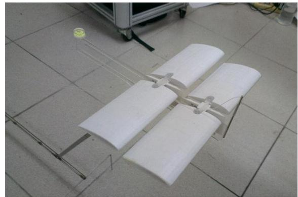
Fig. 8-4 Front wing at  $X_1=6$ cm and the rear wing at position  $X_2=0$ cm.
